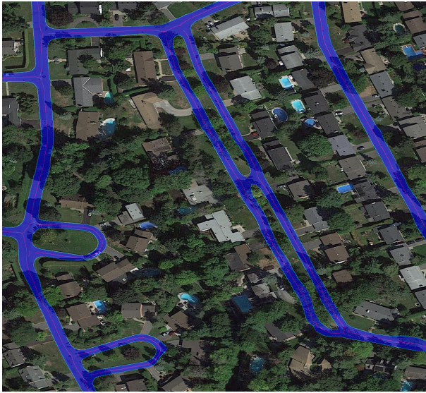
Fig. 1. Road network analysis in complex urban scenes from VHR images at a large scale. Our extracted road surface segmentation (blue), road edges (green), and road centerlines (red) are overlaid over the raw image. Different from previous studies, we pay more attention to the complex urban regions, where shadows and occlusions are very common. Our model predicts pretty good results in these scenes.
